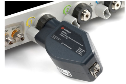
N7004A 33 GHz optical-to-electrical converter
