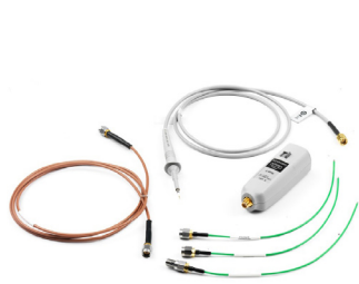
N7020A 2 GHz power rail probe
