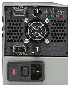
RGA rear panel (with AC power module)
