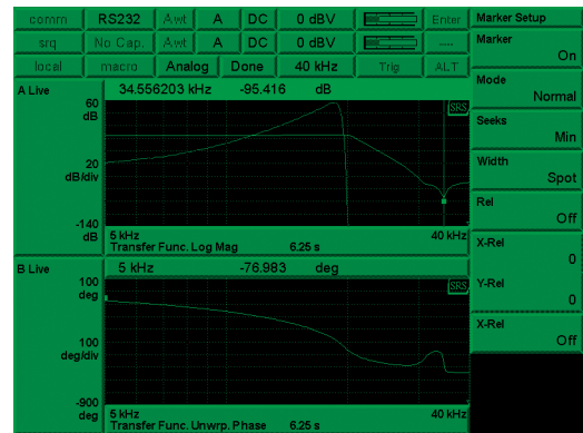
Swept-sine Bode plot of low-pass filter response
